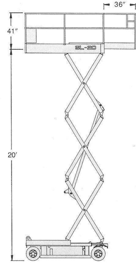
**DANGER:** Models described in this brochure are NON-INSULATED and do not provide electrocution protection from contact with or close proximity to energized conductors which is pointed out on decals and placards attached to the machine.
